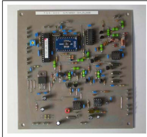
Photograph 1. A board of completed TGS-40C of part implementation
